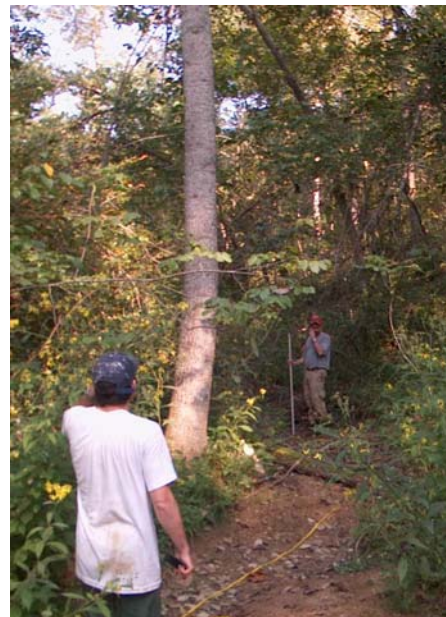
Figure 3-23 Crew members measuring slope of intermittent stream.
