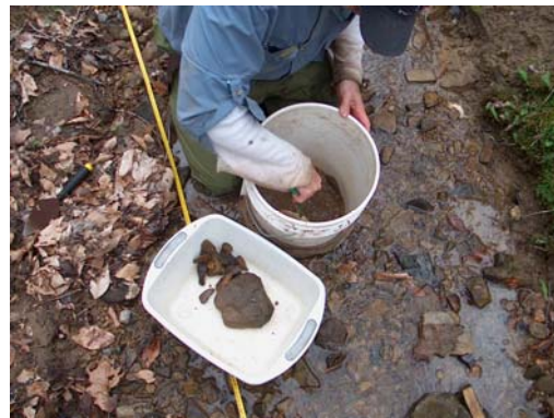
Figure 4-12 Coarse surface substrate set aside in basin for scrubbing.
