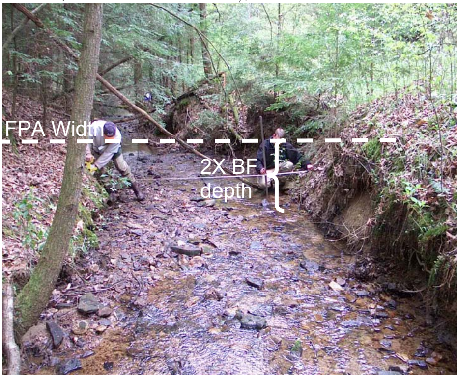
Figure 3-39 Photograph illustrating flood-prone area (FPA) width.
