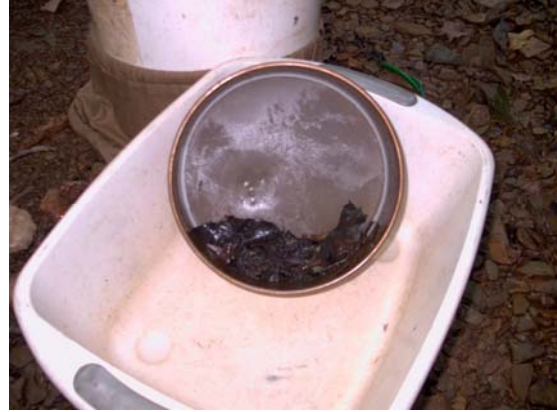
Figure 4-19 Sieve contents condensed for transfer to sample bag.
