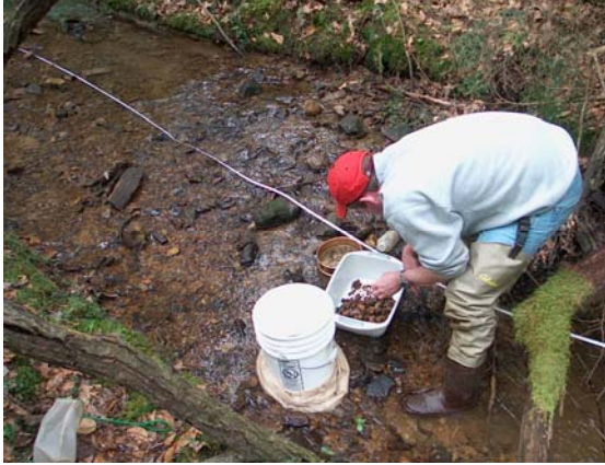
Figure 4-17 Carefully search the basin for heavy-bodied invertebrates that were not transferred to the sieve.
