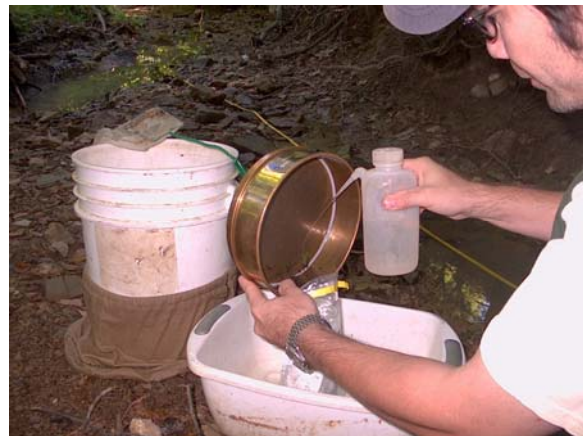
Figure 4-20 Sieve contents rinsed into sample bag (over basin) using ethanol squirt bottle.
